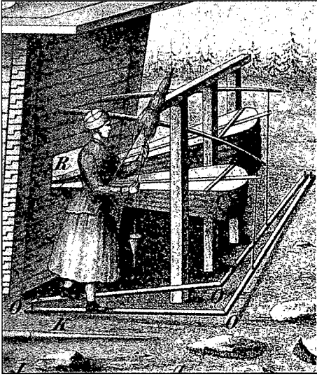
Fig. 1. Woman treading the bellows of an ore blast and simultaneously spinning (Jirlow 1931:114).
