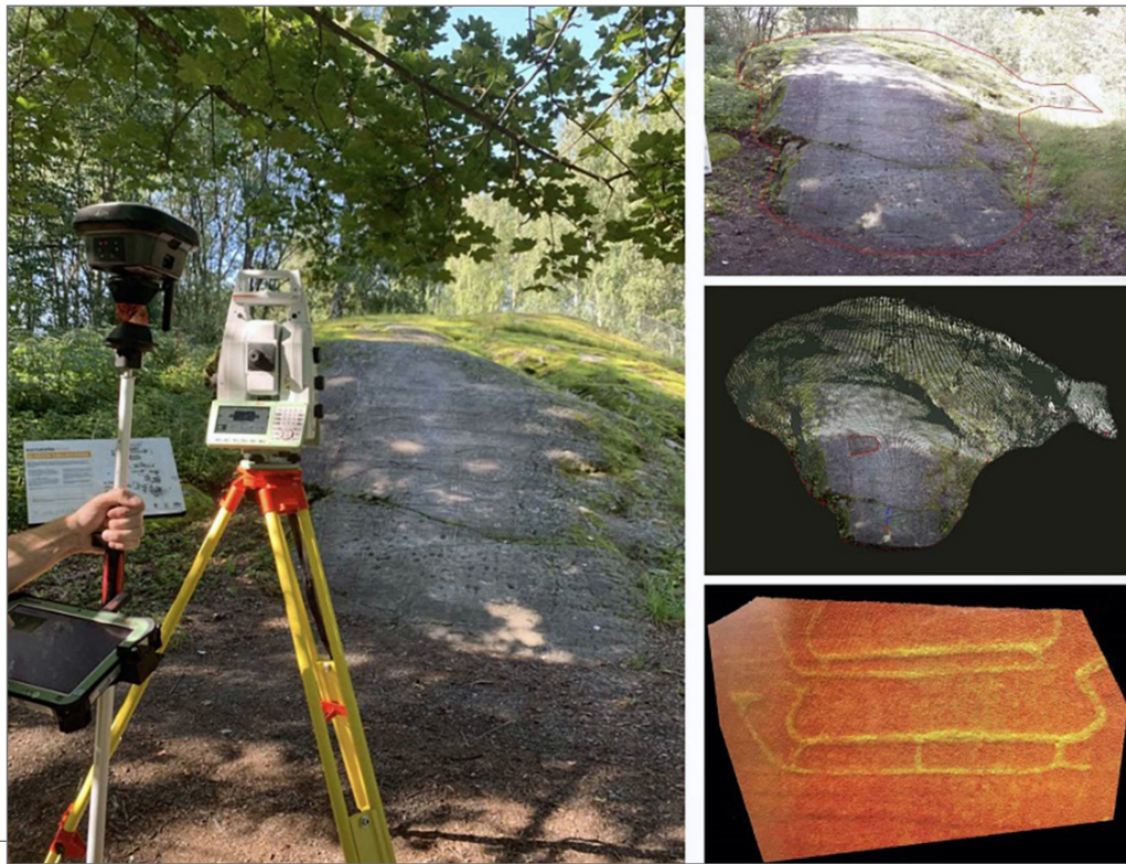
A front scan of the Slagsta hillock (Botkyrka 279) with a Leica MS60. The top right image shows the boundaries of the scan (in red), the middle image shows the resulting point cloud, and the low image illustrates a small section scanned with the highest resolution (1mm).
