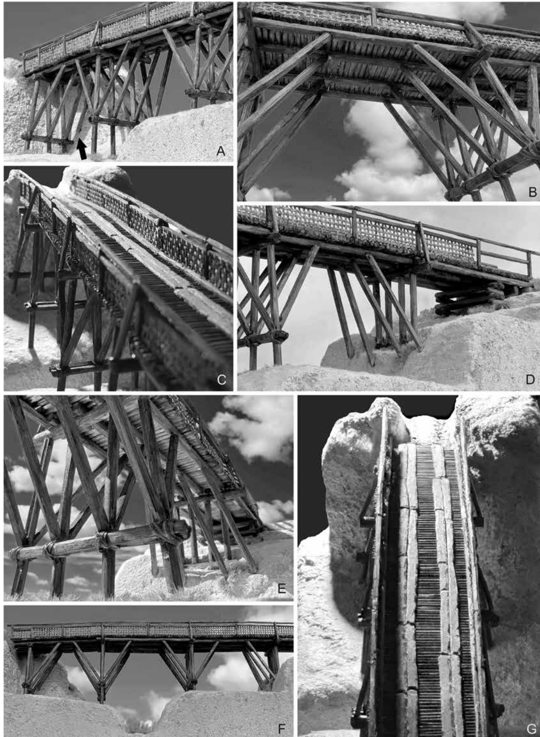
Fig. 13A–G. Spina bridge model reconstruction (scale 1:50) from multiple angles. A: Southern abutment (BA2) showing vertical supports (piers) and the position of the cavity for the inclined strut BH5 (black arrow). B: Central span over the Dogana road, originally c. 10 m high (see F). C: Hypothetical wooden deck with railings and protective planks for iron-wheeled vehicles. D–E: Northern abutment (T4 and BA1) with vertical support (pier) and cavities for inclined struts (BH1–BH4). F: Strut-frame bridge construction with three piers standing on the ground and the cliffside pier, BA1/T4 to the far right. G: Top view of the bridge deck (width c. 3–4 m including rails), connecting to the Spina road. Note the narrowing cliffside (right), which required cavity BH5 to be attached directly into the bedrock instead of relying on a wooden pier (see A). Model and photographs by R. Holmgren. Copyright: Richard Holmgren ARCDoc.
