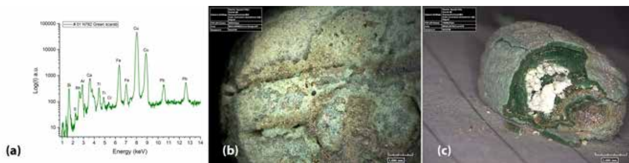
Fig. 47. Non-invasive analysis of scarab N782: (a) XRF spectrum of the base material, (b) micrograph showing corroded surface of the scarab, and (c) micrograph taken after the scarab fell apart exposing its multiple layers and a white material inside (copyrights: Svetlana Gasanova).
