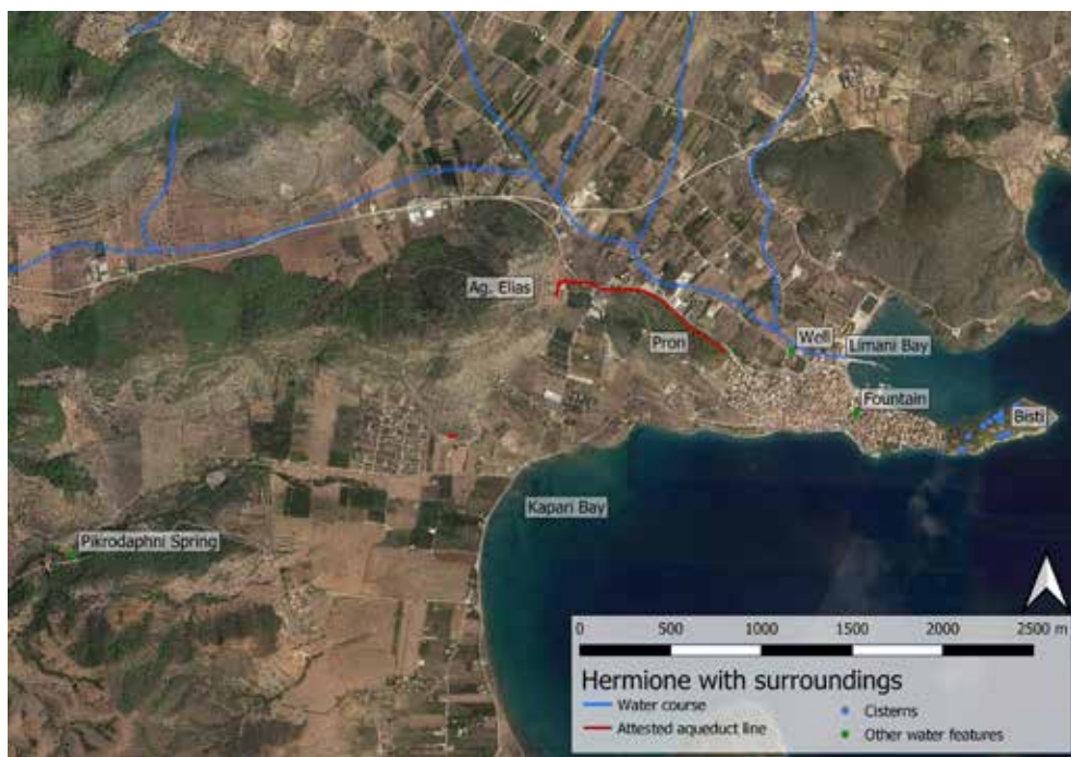
Fig. 1. Map over the area of Hermione with attested sections of the aqueduct (red), the local watercourse (blue), cisterns (blue circles), and other selected water installations (green circles). Illustration by Patrik Klingborg, basemap by Google, ©CNES/Airbus, European Space Imaging, Landsat/Copernicus, Maxar Technologies, Map data 2021.
