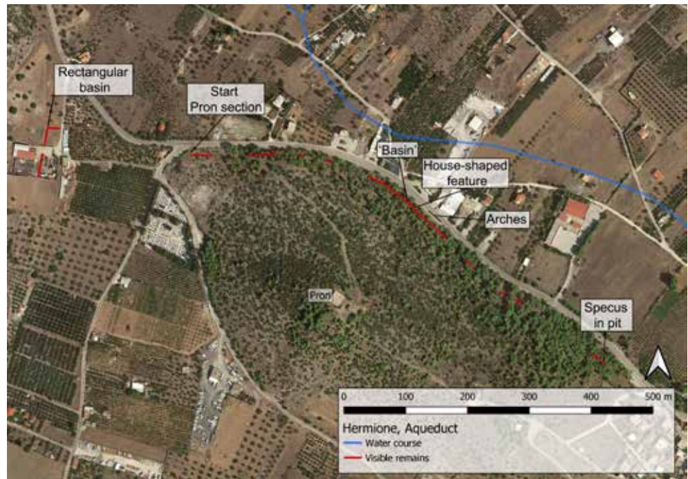
Fig. 2a. Detail of the aqueduct along Pron Hill. Illustration by Patrik Klingborg, basemap by Google, ©CNES/Airbus, European Space Imaging, Maxar Technologies, Map data 2021.
