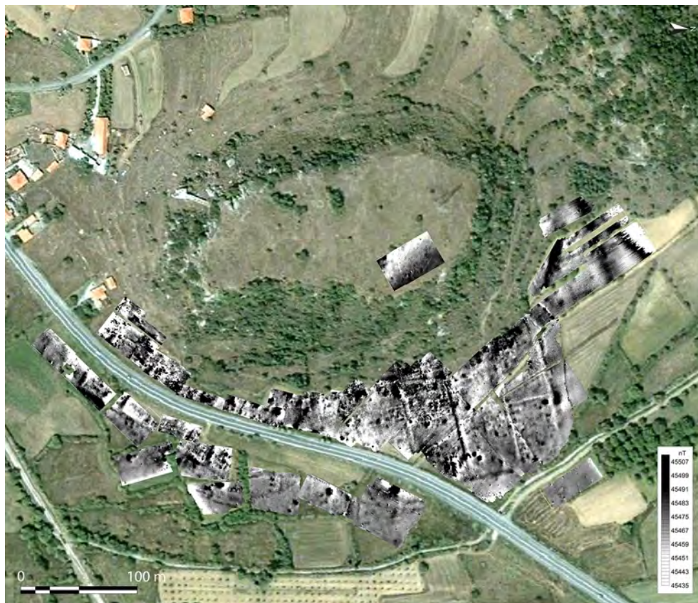
Fig. 1. Grey scale map combined with a Google map showing Asea Paleokastro with the results of the magnetic survey seasons 2007, 2009 and 2012.
