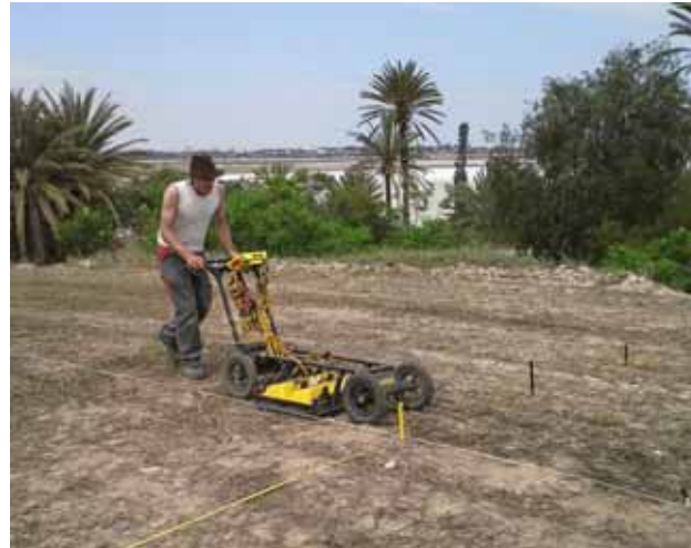
Fig. 34. GPR measurements in Area A with the three-channel 500 MHz system.
